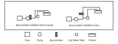
It is recommended the pre-charge be checked annually or anytime the accumulator does not appear to be functioning properly. Temperature and altitude changes can affect the accumulator pressure and performance. Use any standard tire pressure gauge to check pressure.
