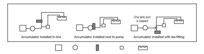
The RACT820-JG has 2 John Guest 3/8" push connect fittings. This tank can only be mounted with through connections. See diagrams in figure 2.
